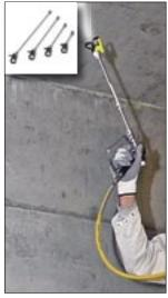
The use of nozzle extensions saves using ladders and scaffolding, extends the radius of action for objects with large surfaces and thus increases working flexibility.
